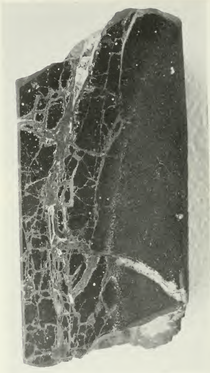
Enlarged view of cut and polished section of a 1-inch core of glassy basalt recovered from near the top of the second layer of the oceanic crust, about 575 feet below the ocean floor under 11,700 feet of water, off Guadalupe Island, April 1961. (Photograph by U.S. Geological Survey.)
