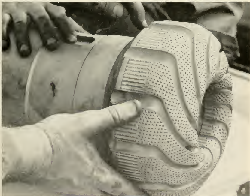
2. The 8½-inch, $8,000 diamond drill bit used in the experimental drilling program for Project Mohole shown aboard the CUSS I .
