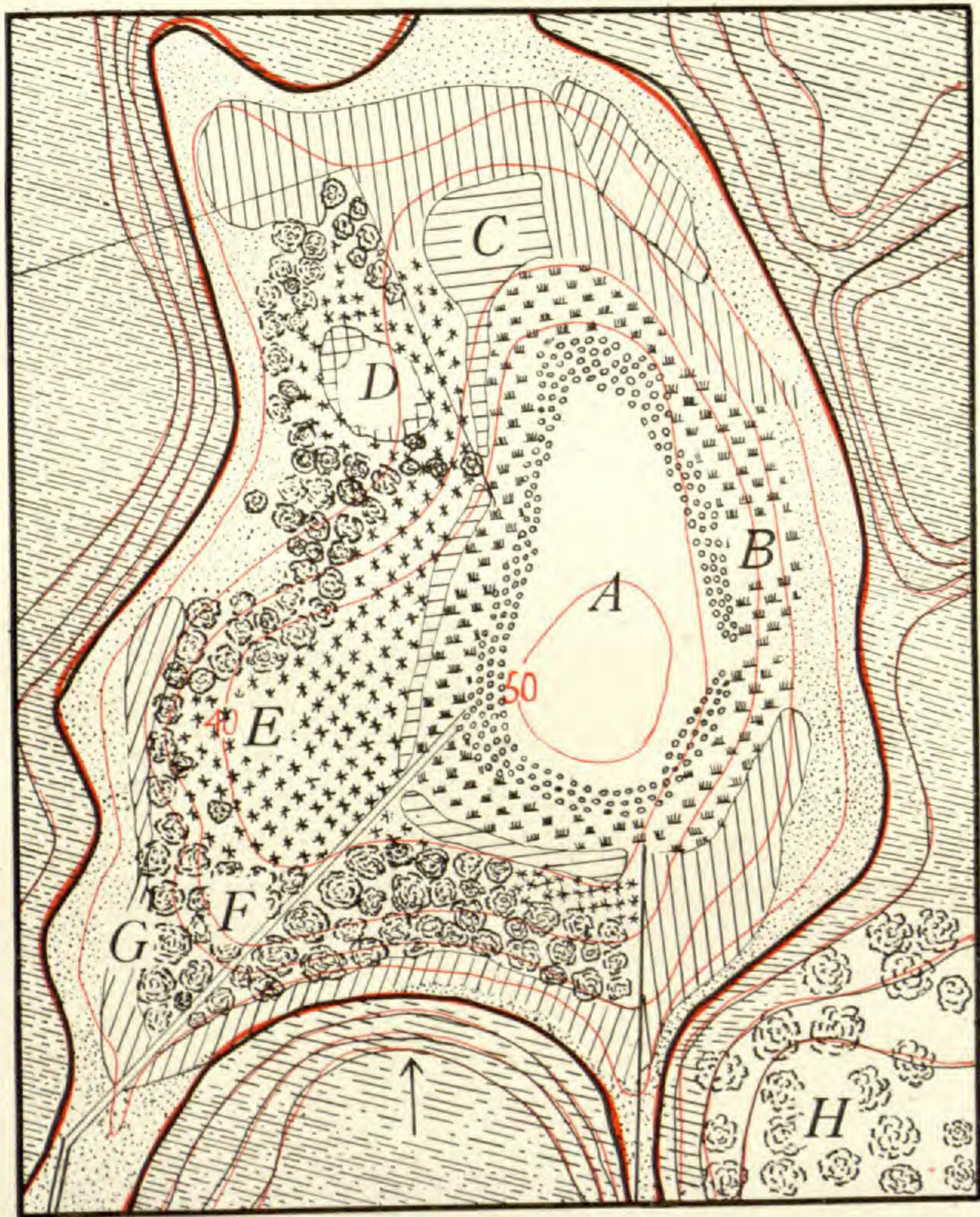
FIG. 1.—First Sister Lake. Contours of the post-glacial lake in red. The heavy line indicates the position of its shore as shown by peat deposit. Scale 1:2880. Contour interval of topography five feet, of hydrography ten feet.
