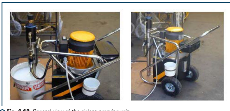
Fig. 4.13 General view of the airless spraying unit
