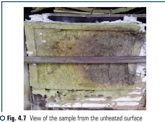
Fig. 4.7 View of the sample from the unheated surface of the steel plate
