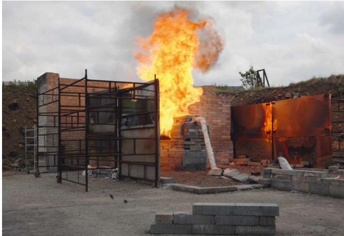
Fig. 4.12 Testing according to the international standard ISO 22899-1:2007 and ISO/CD 22899-2:2009
