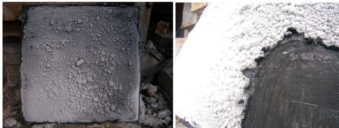
○ Fig. 4.18 General view of "Amotherm Steel Wb" coated steel plate after testing
