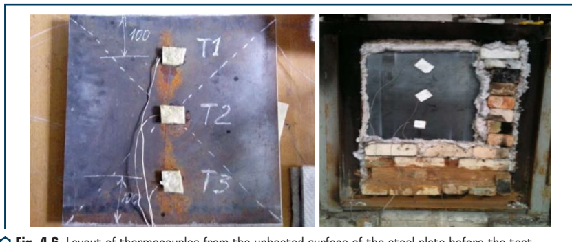
○ Fig. 4.6 Layout of thermocouples from the unheated surface of the steel plate before the test
