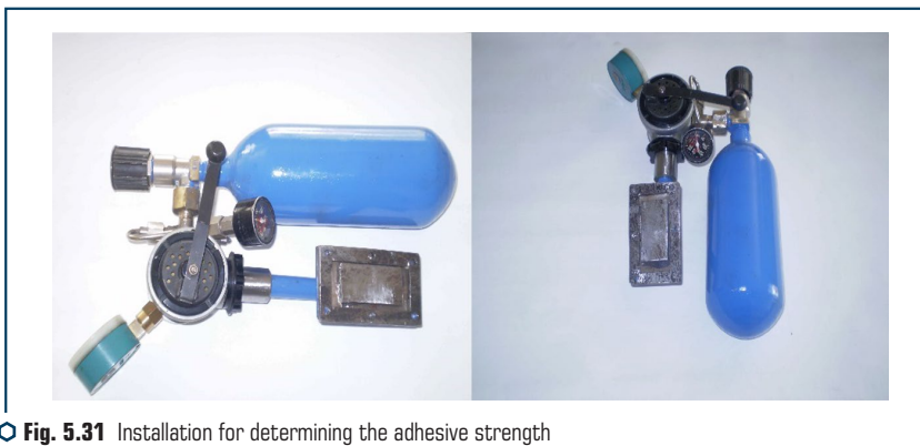
○ Fig. 5.31 Installation for determining the adhesive strength of coatings of fire-retardant steel structures
