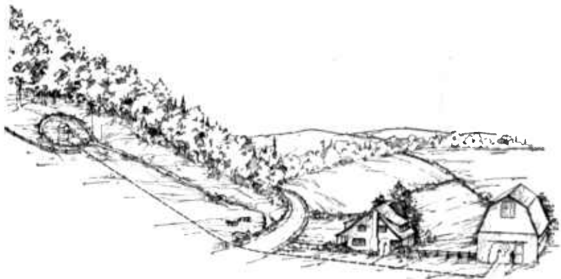
FIG. 12.—Water delivered by gravity (natural flow). Note protection of the spring: a shallow trench on the upper side to divert surface water, and the site inclosed by a fence to keep out stock
