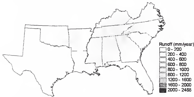
Figure 3. Simulated average annual water yield across the southeastern U.S. with a spatial resolution of 30 m scaled down from a 4 x 4 km 2 resolution.
