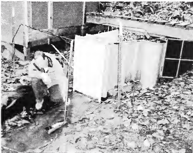
Figure 1. Montana flume with turbidity sensor housing suspended downstream on cable-mounted boom at station Porter in the South Fork of Caspar Creek.
