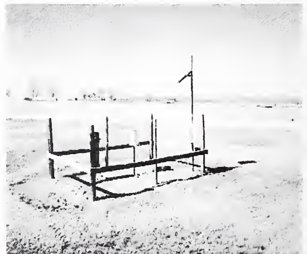
Figure 4. Recording tipping bucket rain gauge and datalogger setup with adjacent standard rain gauge.
