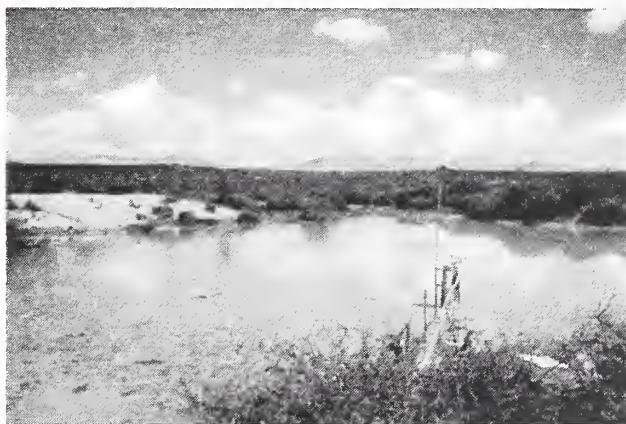
Figure 4. Stage gage for measuring water level at stock Tank 223 on the Walnut Gulch Experimental Watershed.
