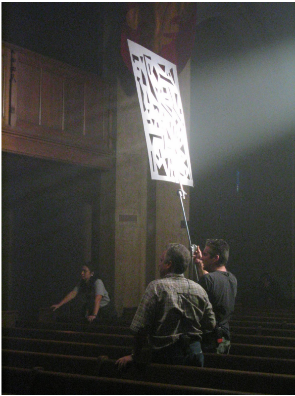
Figure 38 A cookie in action: similar to a gobo but not as close to the light source.
