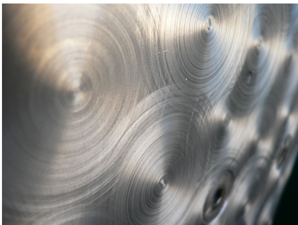
Figure 47 Brushed aluminium. Note the form of the specular highlights, which is far from being round.
