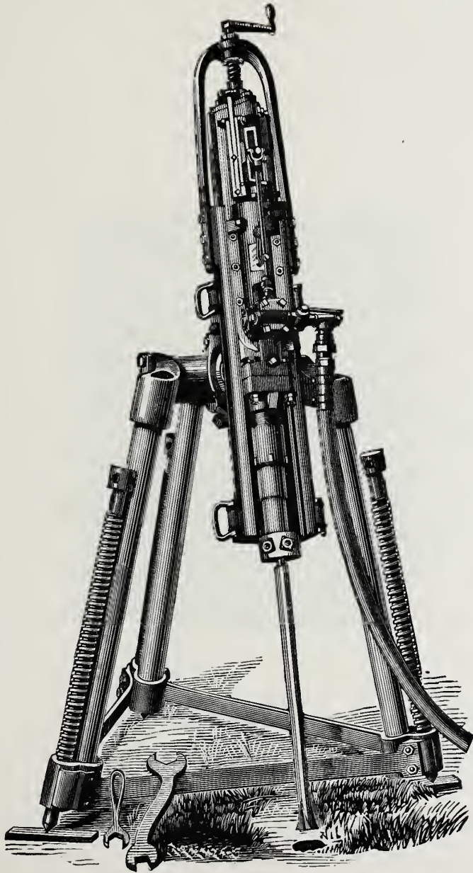
Fig. 1.—Drill Mounted on Iron Tripod for Rock-Cutting.
