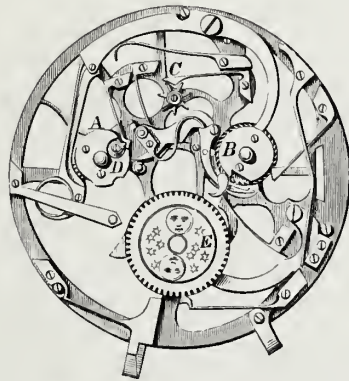
Fig. 2.—Matile Watch—Mechanism of Perpetual Calendar: M. Matile, Locle, Switzerland.
