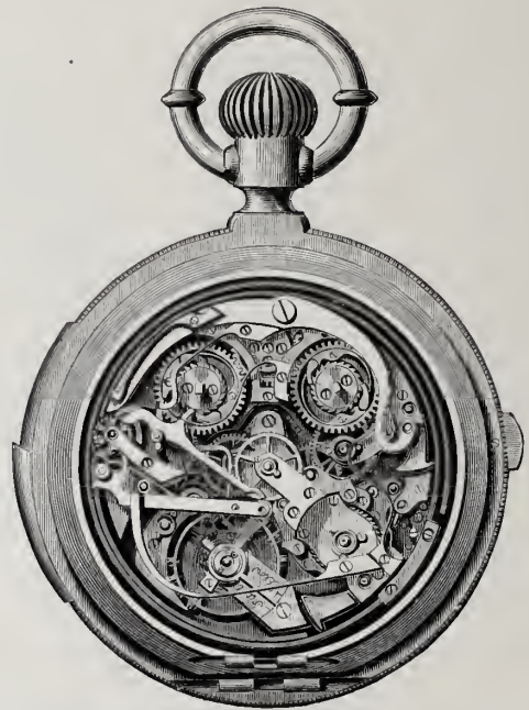
Fig. 4.—Matile Watch—Main Train and Mechanism of the Chronograph: M. Matile, Locle, Switzerland.
