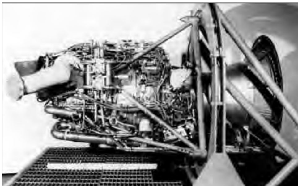
The XLR99 on a maintenance stand. The engine used ammonia (NH 3 ) as fuel and liquid oxygen (LOX) as the oxidizer. The XLR99 required a separate propellant, hydrogen peroxide, to drive its high-speed turbopump—the Space Shuttle Main Engine uses the propellant itself (LH 2 or LO 2 , as appropriate) to drive the turbopumps. (AFFTC via the Tony Landis Collection)
