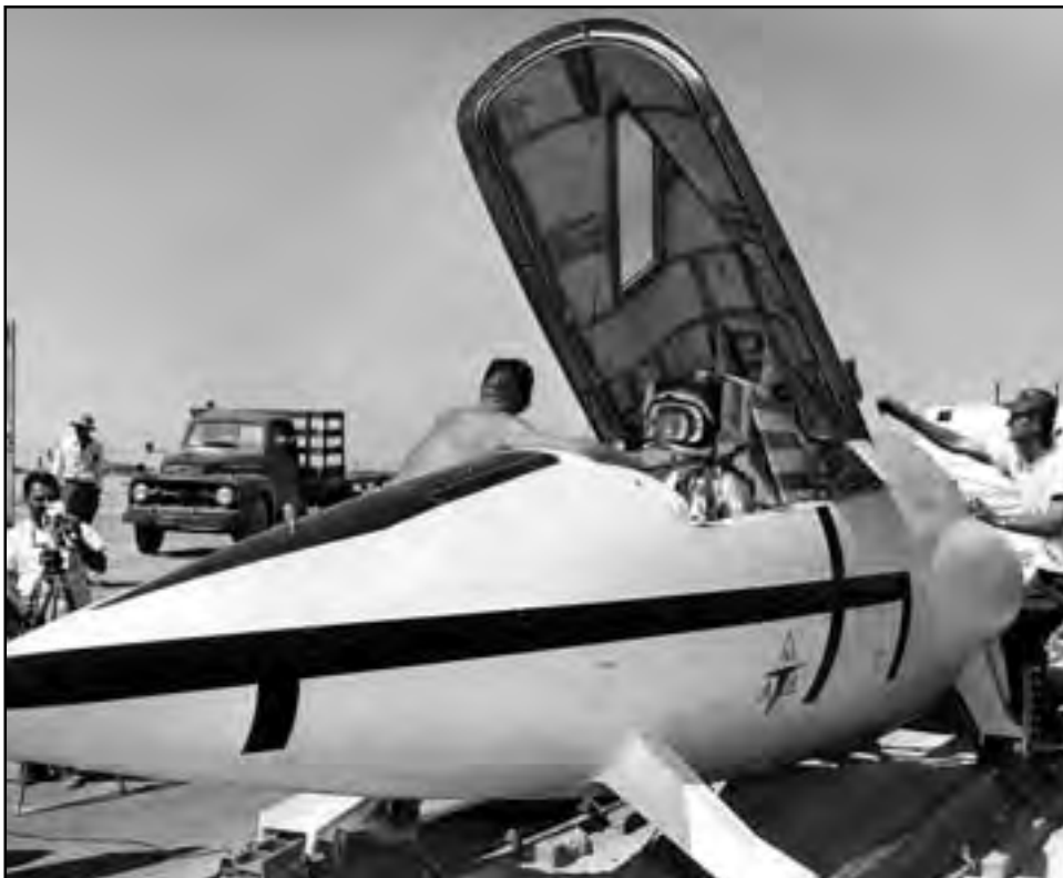
A great deal of X-15 research did not involve the actual aircraft. Here a rocket sled is being used to test the ejection system. (Jay Miller Collection)
