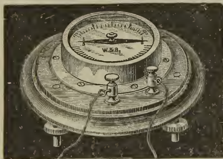
FIG. 152.—A HORIZONTAL MILLIAMPERE-METER. (After the Thistleton pattern.) The screw-feet allow of adjustment so as to insure a perfect leveling of the instrument. It is then revolved so that the needle (which will point north) rests at the zero point of the dial. Reversal of the current diverts the needle to the opposite side. One of the rheophores shown goes to a binding-post of the battery, and the other to one of the electrodes employed upon the patient. This instrument is very delicate, but the eye has to look down upon the dial in order to observe the deflection of the needle. If the instrument is placed lower than the eye, this objection is not serious. With it it is easy to detect small fractions of a milliampère of current, and it is much less expensive than a good vertical galvanometer and more accurate than most of those offered to the profession. I do not recommend them for measuring very high currents.
