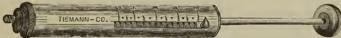
FIG. 63.—BEARD'S PIESMETER.—This instrument consists of a spring in a tube that resists pressure made upon the piston. A scale indicates the amount of pressure upon the spring. It is employed to determine the degree of sensitiveness to pressure in different parts of the body. The forehead, tongue, and cheek are the most sensitive to pressure; the least so are the backs of the thighs and legs.
