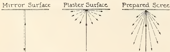
Figure 4—Types of screen surfaces. The relative amount and direction of the reflected light is indicated by the broken lines.
