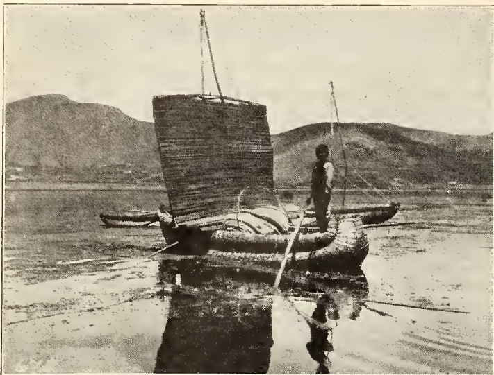
A reed boat, known to the natives of South American countries as "balsa," on Lake Titicaca, Bolivia.
