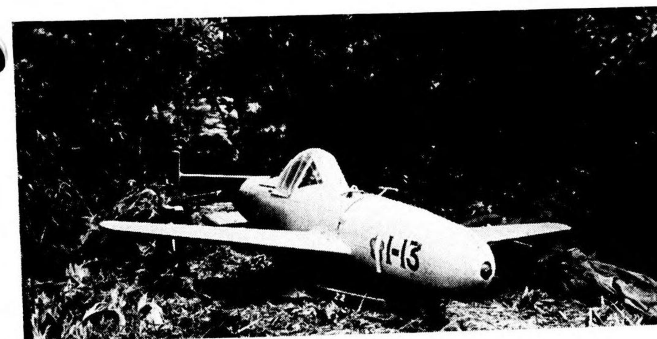
Captured BAKA —Here a BAKA is pictured in a clearing on Okinawa showing general construction and appearance. Note a metal eye in front of cockpit for attaching to parent-plane.
