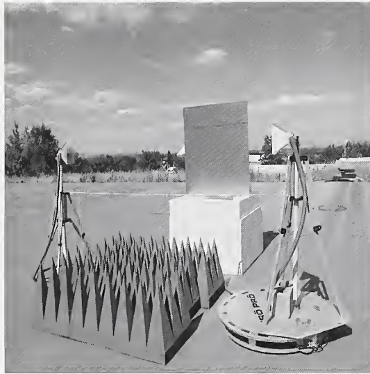
Scattering object testing at NIST OATS facility
