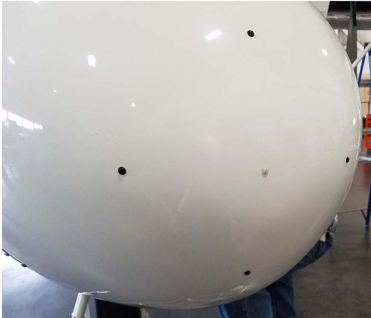
Figure 5. Nose of NPS Twin Otter where Radome tube intakes are evident (black circles)
