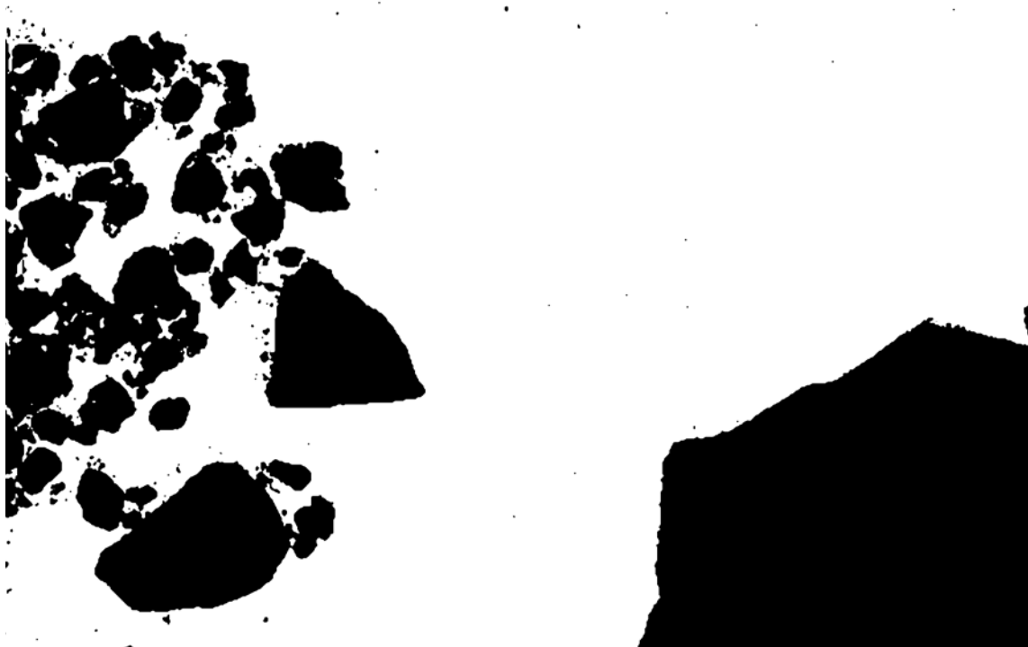
Figure 23. Example output from dl_tools, a mask of ones and zeros for use in the ML model, ones (zeros) are depicted in black (white) and represent ice (water)
