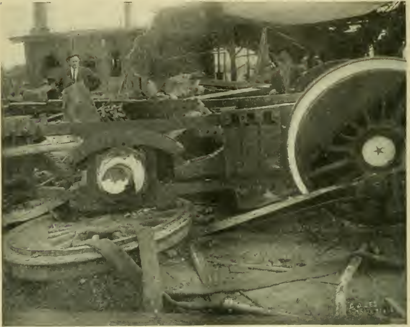
FIG. 3. DRIVER BLOWN FROM AXLE.
