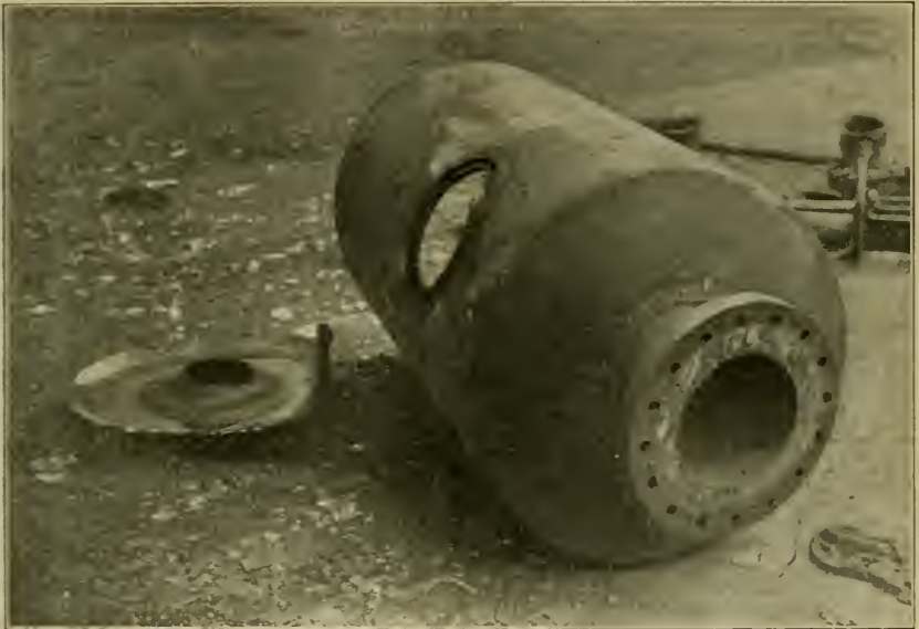
FIG. 4. THE WRECKED SEPARATOR.
