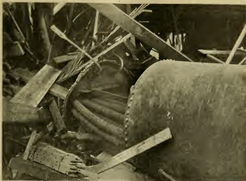
FIG. 1.— SHOWING THE EXPLODED BOILER.
