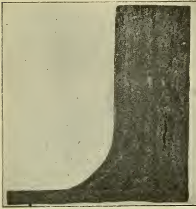
FIG. 2.—SECTION OF STEAM PIPE AND FLANGE. (ETCHED.)
