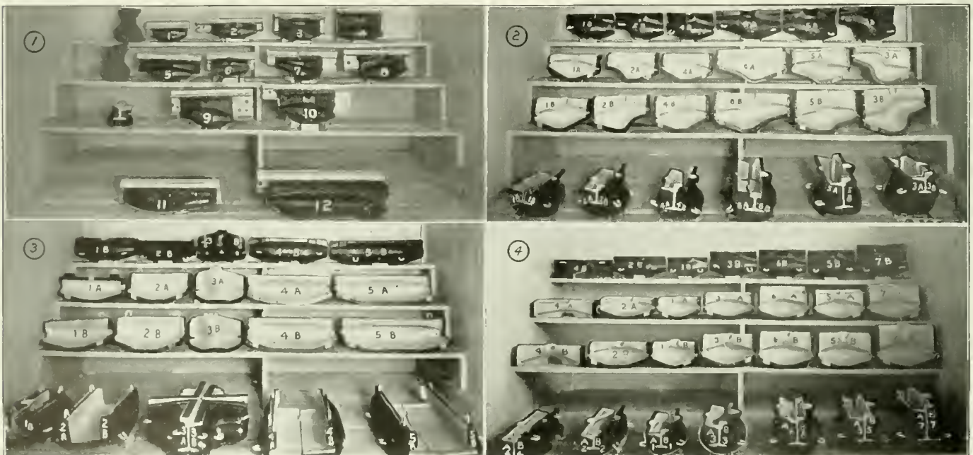
CAST-WELDED JOINTS AND MOLDS, CHICAGO CITY RY.
