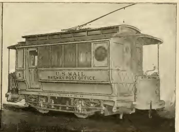
FIG. 1—OLD PASSENGER CAR RECONSTRUCTED FOR A MAIL CAR IN BROOKLYN. FIG. 2.
