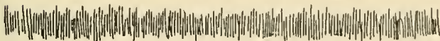
Fig. 3. One Cast-Iron Fly-wheel 5½ feet diameter, and one Tangent-Spoke Fly-wheel 10 feet diameter Weight of Rims 1470 + 2600. = 4070 lbs Total Weight of Wheels 1670 + 2900 = 4570 lbs Thirteen impulses per minute.
