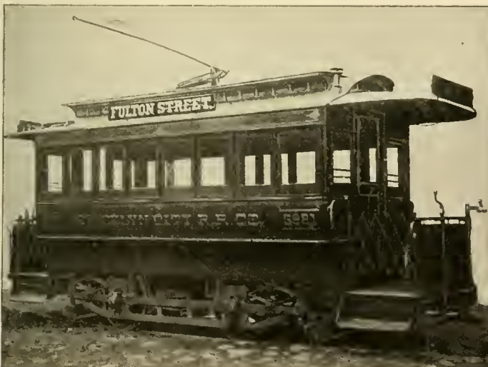
FIG. 1—OLD PASSENGER CAR RECONSTRUCTED FOR A MAIL CAR IN BROOKLYN. FIG. 2.
