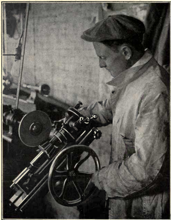
Fig. 163.—Grinding a formed cutter on a Brown & Sharpe formed-cutter grinding attachment.
