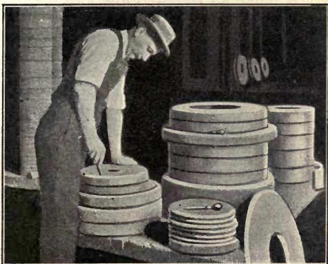
Fig. 15.—Grading grinding wheels by the hand-test method.
