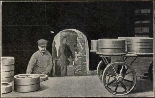
Fig. 12.—Loading a grinding-wheel kiln.
