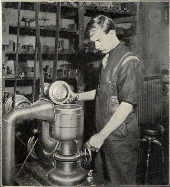
Fig. 85.—Grinding piston rings on a Heald ring and surface grinder.
