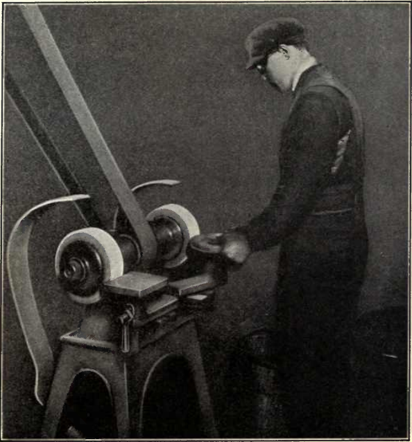
Fig. 56.—These guards are inadequate and invite disaster.
