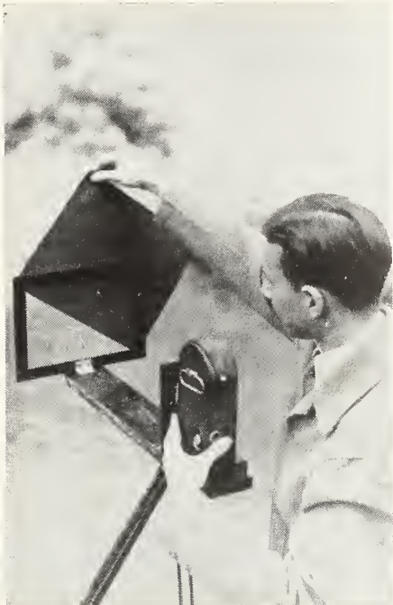
WIPE is made by sliding black cardboard mask diagonally across holder, producing effect illustrated at the right.
