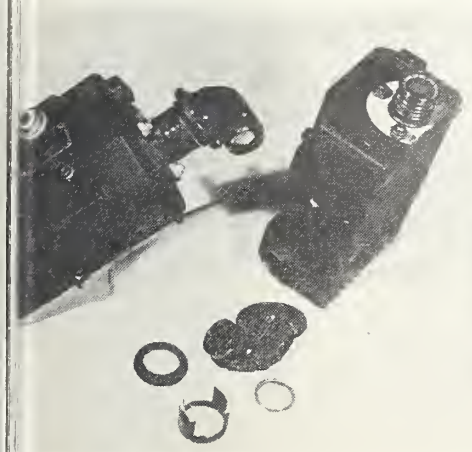
● SALVAGED camera has lens erector system, as shown here, it should be removed, leaving only the lens.
