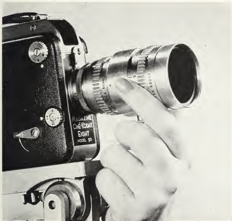
FOCAL LENGTH of a lens determines the size of the image on the film. This 50mm. lens on an 8mm. camera would give four times the image size obtainable with the ordinary 13mm. lens. At f 1.6, the opening in the lens would pass approximately twice the amount of light it would at f 2.
