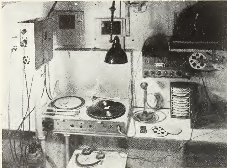
PROJECTION setup shows the author's home-built mechanism. On the turntable at the left can be seen the ring that surrounds the plate, holding the record slightly above the revolving disc until it is automatically dropped at the proper moment. In this picture, the ring has dropped below the plate.
