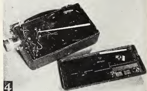
BACKWIND construction is shown in this series of photos and the diagram below. Fig. 1—The knurled screw in upper left hand corner of camera case must be turned so white dots are adjacent before starting to backwind. Fingers of left hand are in position to depress camera starter button as handle is turned. Fig. 2—Camera with cover removed to show position film takes after backwinding. Fig. 3—Parts required (left to right) spring, winding handle cell assembly, sprocket driver (shadow shows pin arrangement), winding handle, stud. Eccentric cam is in upper right hand corner of camera cover. Camera case bushing is in place. Fig. 4—Upper left toothpick points to top of phonograph needle which, when depressed, lifts spring clip to disengage it from sprocket hold, allowing film to wind back. Middle toothpick shows sprocket with holes drilled. Right toothpick points to eccentric cam in position. Sprocket driver is also shown. Spring and cell assembly in place. Fig. 5—Closer detail of phonograph needle and holes in sprocket.
