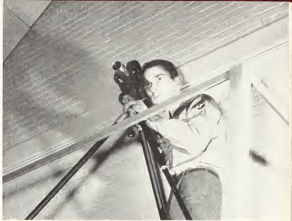
● HIGH IN the University's gymnasium Richard Thiriot focuses his Bell & Howell 70-DA on a critical basketball play taking place below. Analysis films of this type are shot with a telephoto lens at 32 frames per second. Thiriot gets adequate exposure using Ansco Triple-S pan film and a stop of f/1.6.
