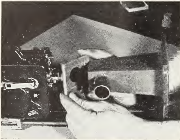
AT THE small end of the matt box is an auxiliary lens holder. Here it is being properly aligned before cementing to matt box housing. It will take filters or spectacle lens auxiliaries.
