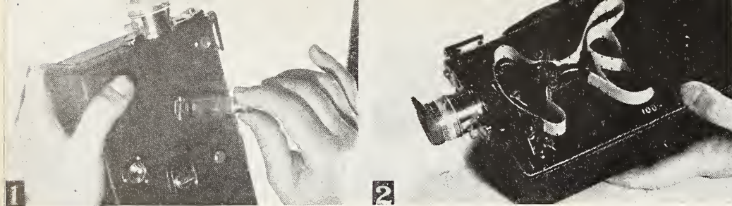
BACKWIND construction is shown in this series of photos and the diagram below. Fig. 1—The knurled screw in upper left hand corner of camera case must be turned so white dots are adjacent before starting to backwind. Fingers of left hand are in position to depress camera starter button as handle is turned. Fig. 2—Camera with cover removed to show position film takes after backwinding. Fig. 3—Parts required (left to right) spring, winding handle cell assembly, sprocket driver (shadow shows pin arrangement), winding handle, stud. Eccentric cam is in upper right hand corner of camera cover. Camera case bushing is in place. Fig. 4—Upper left toothpick points to top of phonograph needle which, when depressed, lifts spring clip to disengage it from sprocket hold, allowing film to wind back. Middle toothpick shows sprocket with holes drilled. Right toothpick points to eccentric cam in position. Sprocket driver is also shown. Spring and cell assembly in place. Fig. 5—Closer detail of phonograph needle and holes in sprocket.
