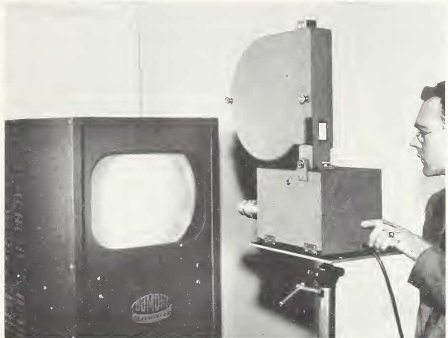
• A flip of a switch starts the new Kodak TV 16mm. television recording camera developed by Eastman Kodak Company at Rochester, N. Y. The Camera produces movies directly from face of the television monitoring tube, which can be used as medium for rebroadcast of programs, air-checks, and for movie screen program material.
