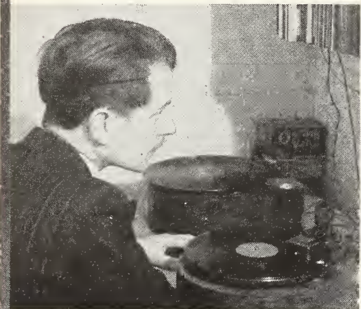
TWIN turntables provide incidental music and special effects for silent films projected in the theatre. Special recordings are made here, too.
