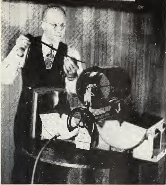
● TYPICAL of the amateur who processes his own movie film is Karl Brueckner of Milwaukee, who designed and built his own equipment shown here. Outfit handles 50 feet of film at a time.
