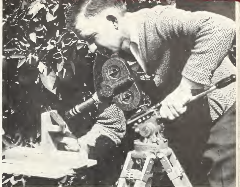
● ULTRA CLOSEUP cinemicrography is accomplished through use of 3-inch extension tube. Here author is adjusting the moveable stage to bring subject matter within range of the camera, before making final focusing adjustments via the Goerz Reflex Focuser inserted ahead of lens.
