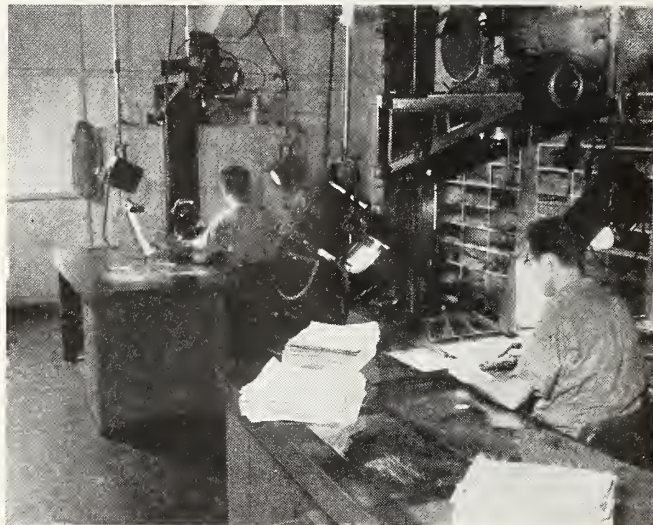
CARTOON photography utilizes overhead camera aimed at scene displayed on table below. This is how MGM's "Senior Droopy" was made, drawings being combined with live-action scenes.
