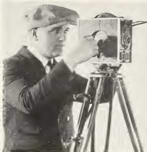
GRANDFATHER of today's home movie camera is this Cine-Kodak Model A, introduced in 1923. It was hand cranked.
