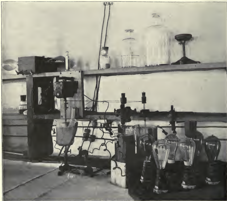
DEPARTMENT OF CHEMISTRY—IODOFORM FROM ACETONE BY ELECTROLYSIS, USING TWO CATHODES AND A ROTATING ANODE
