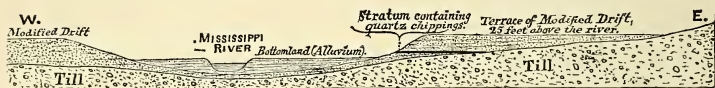
FIG. 73.—Section across the Mississippi Valley at Little Falls, Minnesota, showing the stratum in which chipped quartz fragments were found by Miss F. E. Babbitt, as described in the text (Upham).
