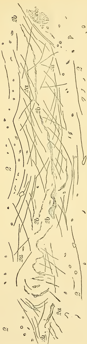
FIG. 48.—Enlarged section of the shelly sand and surrounding clay at B in preceding figure. Scale, 4 feet to 1 inch. EXPLANATION.—2. “Basement” boulder-clay. 2a. Pure compact blue and brown clay of aqueous origin, bedding contorted and nearly obliterated, but the mass is cut up by shearing planes. 2b. Irregular seam, and scattered streaks, of greenish-yellow sand with many marine shells. 2c. Patch of pale-yellow sand, different from 2b, without trace of fossils.
