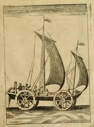
The Body of it being somewhat like a Boat, moving upon 4 Wheels of an equal Bigness, with two Sails like those in a Ship; there being some Contrivance to turn and steerit, by moving a Rudder which is placed beyond the two hindmost Wheels; and for the stopping of it, this must be done, either by letting down the Sail, or turning it from the Wind.
