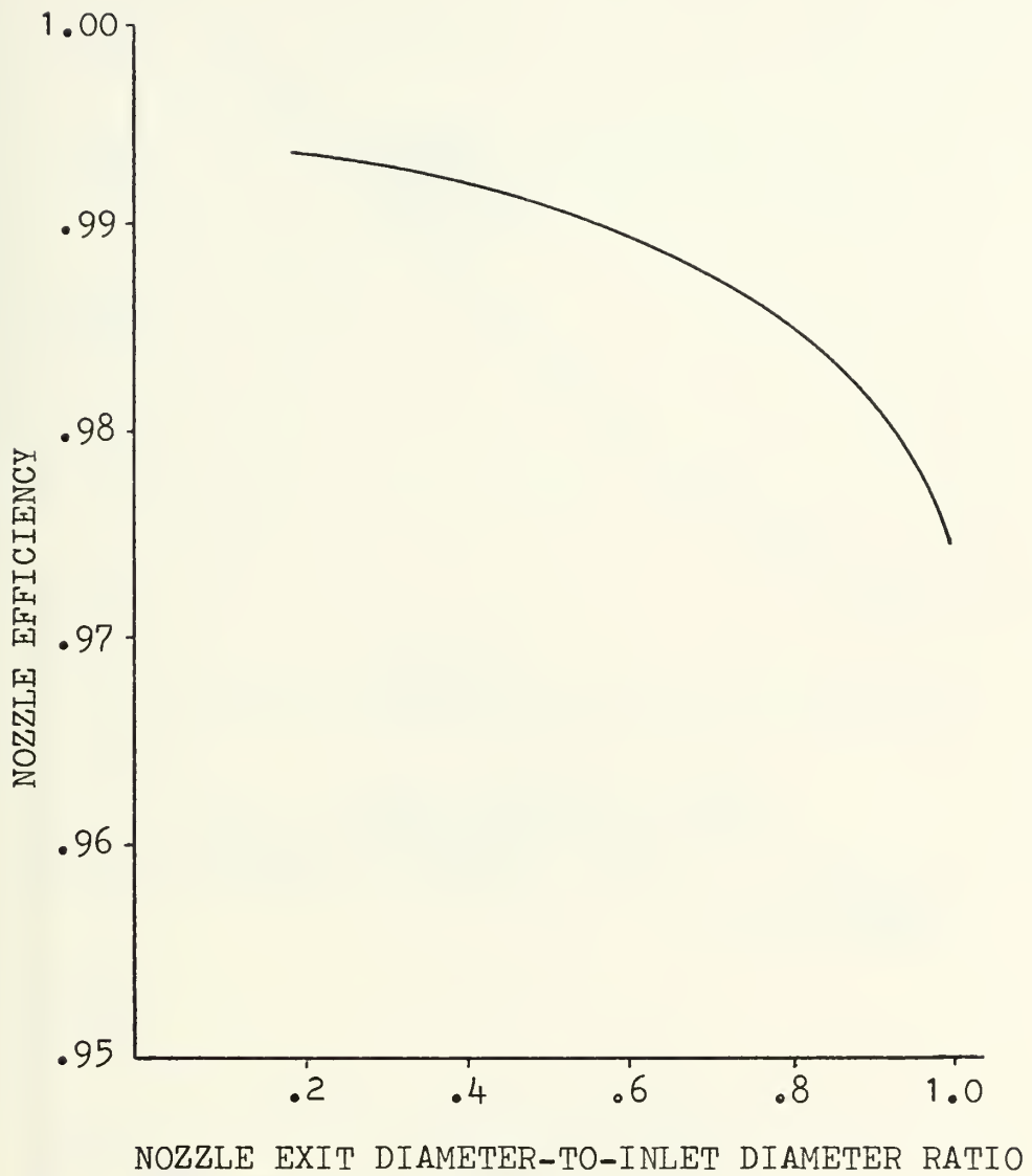
Figure 5 - VARIATION OF NOZZLE EFFICIENCY WITH THE NOZZLE EXIT DIAMETER-TO-INLET DIAMETER RATIO (d/D) FOR A LONG RADIUS NOZZLE
