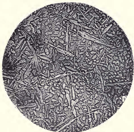
PHOTOGRAPH 33. CUPRO-ALUMINIUM. CAST AND QUENCHED FROM 500°. × 60.
