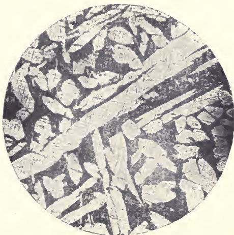
PHOTOGRAPH 32. CUPRO-ALUMINIUM. CAST AND ANNEALED AT 900^{\circ} . \times 225 .
