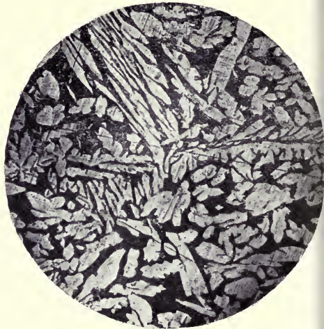
PHOTOGRAPH 6. CUPRO-ALUMINIUM. FORGED AND SUBSEQUENTLY ANNEALED AT 700°. × 225.
