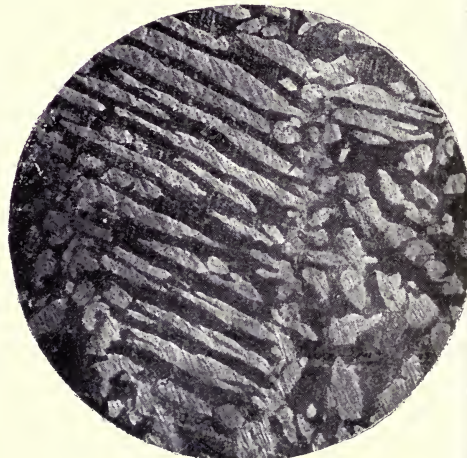
PHOTOGRAPH 12. CUPRO-ALUMINIUM. FORGED AND SUBSEQUENTLY QUENCHED FROM 600°. × 225.
