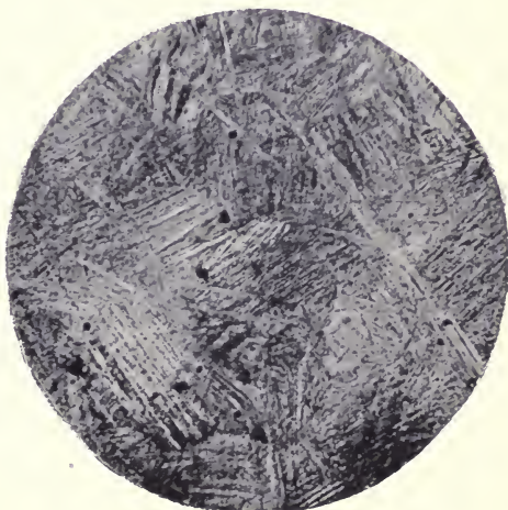
PHOTOGRAPH 35. CUPRO-ALUMINIUM. CAST AND QUENCHED FROM 700°. × 60.
