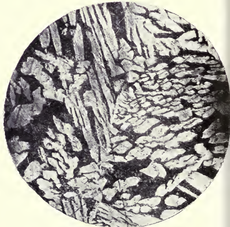
PHOTOGRAPH 8. CUPRO-ALUMINIUM. FORGED AND SUBSEQUENTLY ANNEALED AT 900°. × 225.
