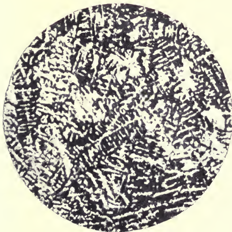
PHOTOGRAPH 1. ALUMINIUM INGOT. CHILL CAST. × 40. (Robert J. Anderson.)
