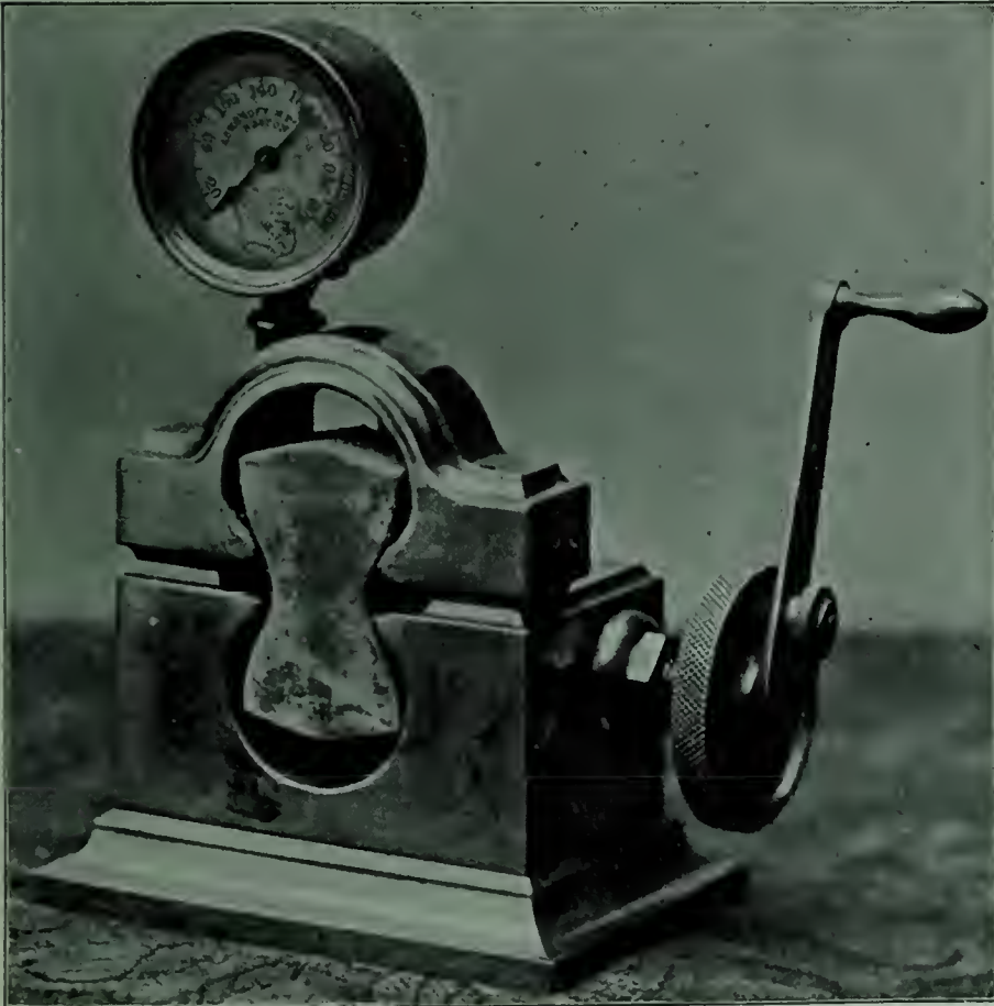
CUMMINGS HYDROSTATIC CEMENT TESTER, CAPACITY 300 POUNDS.
