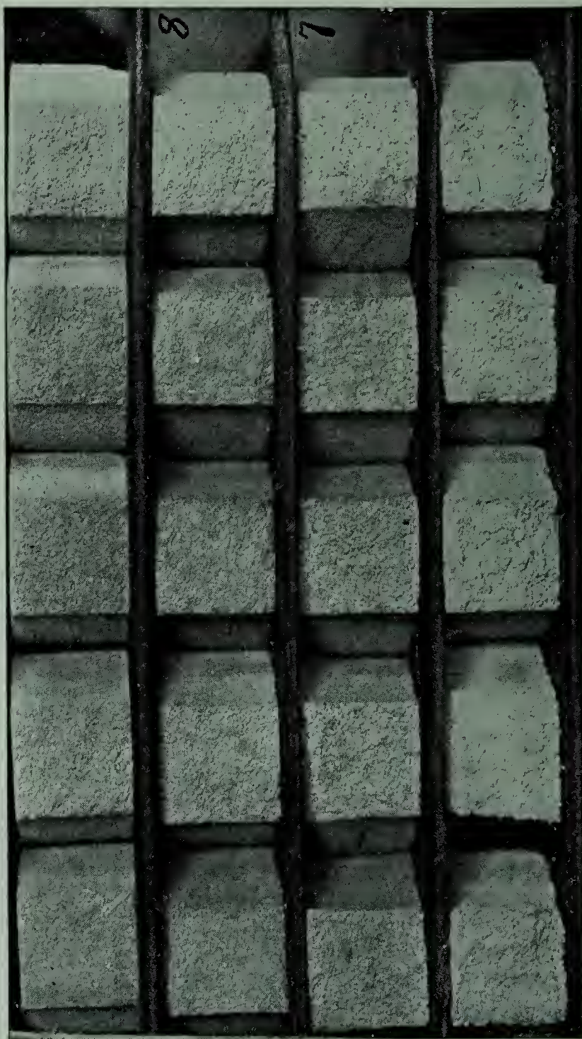
View of fractured sections of Cement Briquettes of the same composition and molded by the same method but by different persons. Numbers on right of horizontal rows indicate number of Laboratory where briquettes were made.
