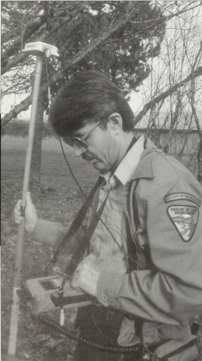
A BLM engineer uses a global positioning system (GPS) unit in Oregon.
