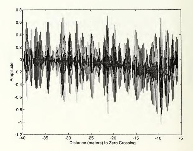
Figure 7.1 Mean filtered point charge response with colored noise. The noisy point charge response is presented in Figure 7.
