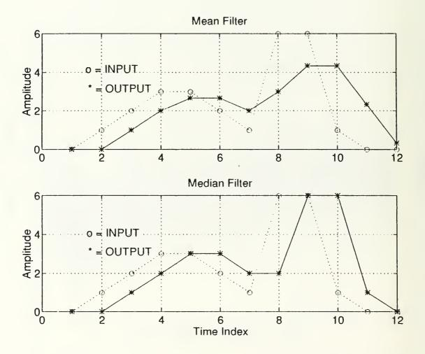
Figure 4 Input/output relationships for the mean and median filter of length three (L = 3). The input data sequence length is 112 (N = 112). The output stays equal to zero until the filter is completely initialized.
