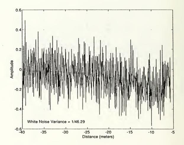
Figure 9 Point charge response with additive white noise, SNR = 4.86 dB.
