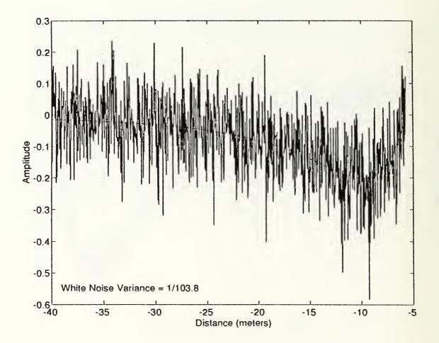
Figure 8.1 Combination mean/median filtered noisy point charge response. The noisy point charge response is presented in Figure 8. The threshold point is represented by (\*), and the zero crossing/fuzing point is represented by (o)
