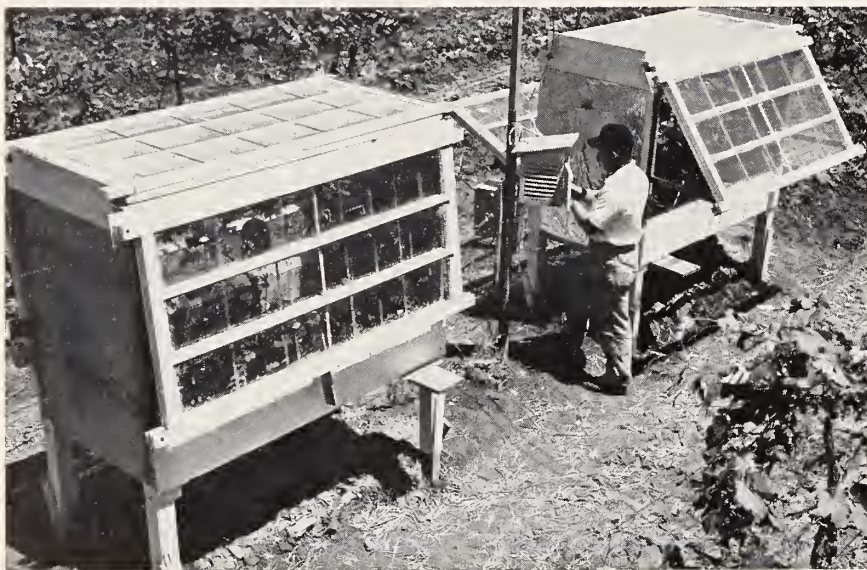
Fruits are grown in the field under controlled environment at the Pennsylvania Experiment Station. With devices such as this, daily growth rhythms of grapes, cherries, and apples have been established. It was noted that such fruits tend to shrink during the forenoon.
