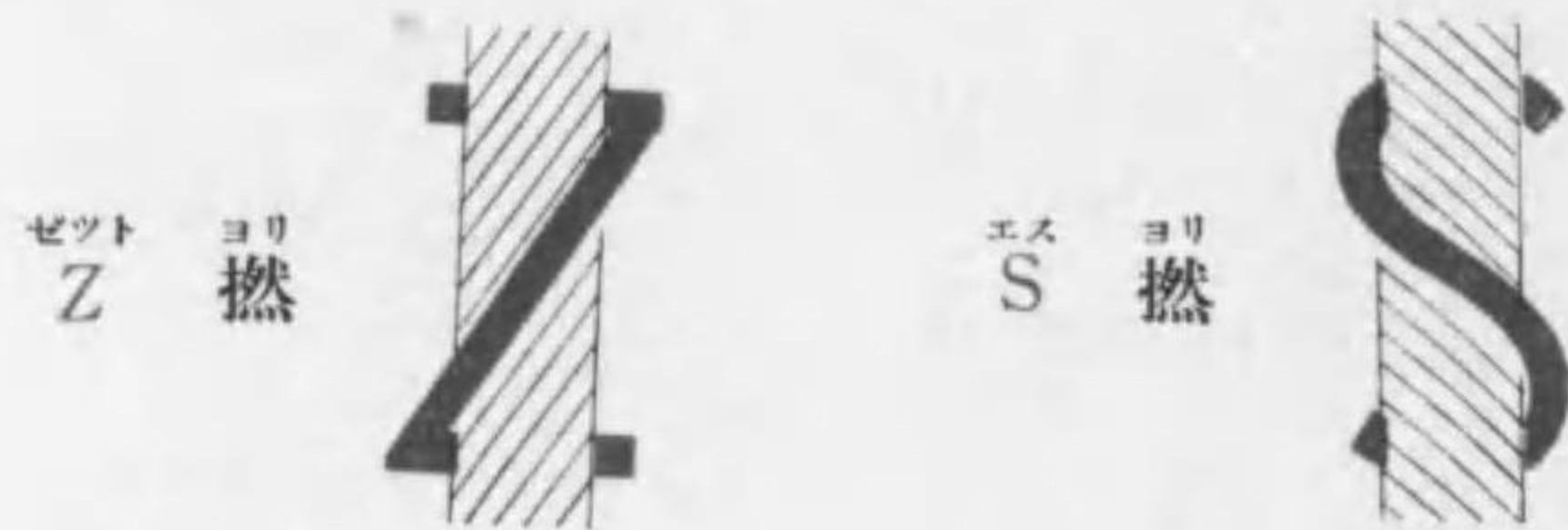
(左撚、並撚、Right-hand Lay) (右撚、逆撚、Left-hand Lay)
