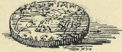
FLAN STAMPED FROM SHEET-METAL. FIG. 12.
