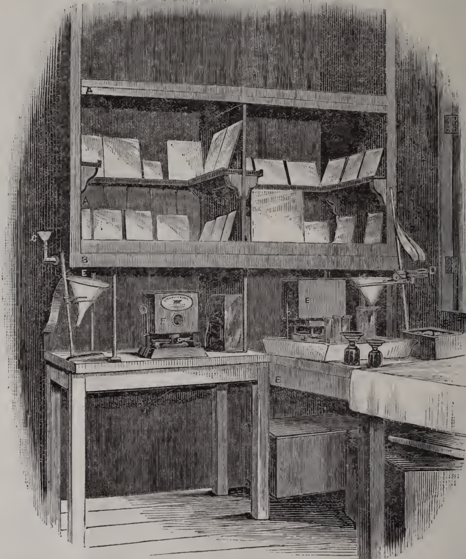
A, wooden cupboard with shelf or shelves, midway, or any other distance up; B, tin or zinc boiler; C, funnel for supplying water to boiler; D, vent for the escape of steam; E, iron framework, upon which boiler and cupboard rest, hollow underneath; F, a paraffin lamp, or, preferably, a Wright and Butler's cooking stove; a thick curtain, to let down wholly or partially, is required, to exclude outer air, and retain heat.
