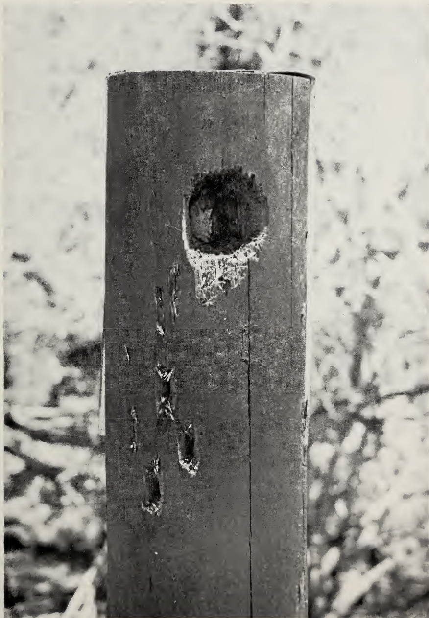
FIG. 3. A flat metal plate has been inserted into a groove cut into the top of this creosoted pine fence post. A woodpecker has drilled a hole to the plate. Small holes are scattered about near the large hole.
