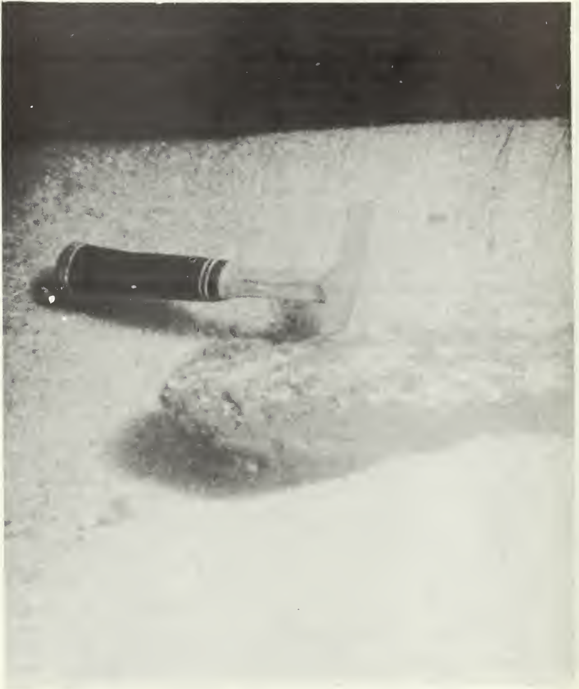
Figure 12. Photo of a Broken Piece of Silty Clay Containing Coarse Biogenous Material
