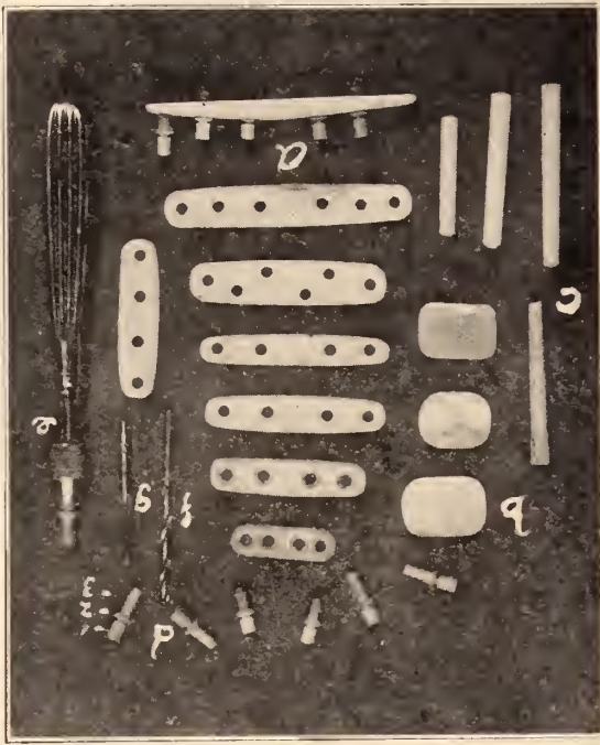
Fig. 1. Showing plates, screws, and pins made of ox-bone. (a) Plates of varying sizes and thickness. (b) Flat plates for skull repair. (c) Pins, of varying sizes. (d) Screw with 1, partially detached handle, 2, counter sunk head, and 3, machine screw thread. (e) Screw holder, showing manner screw is held. (f) Drill. (g) Tap.
