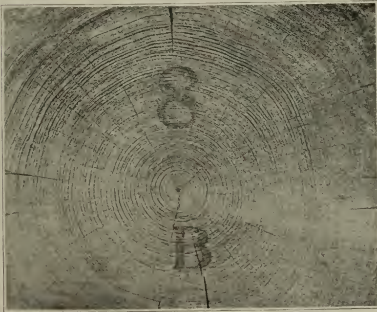
END SECTIONS OF BEAMS FROM LONGLEAF PINE, PHOTOGRAPHED BEFORE TESTING.
