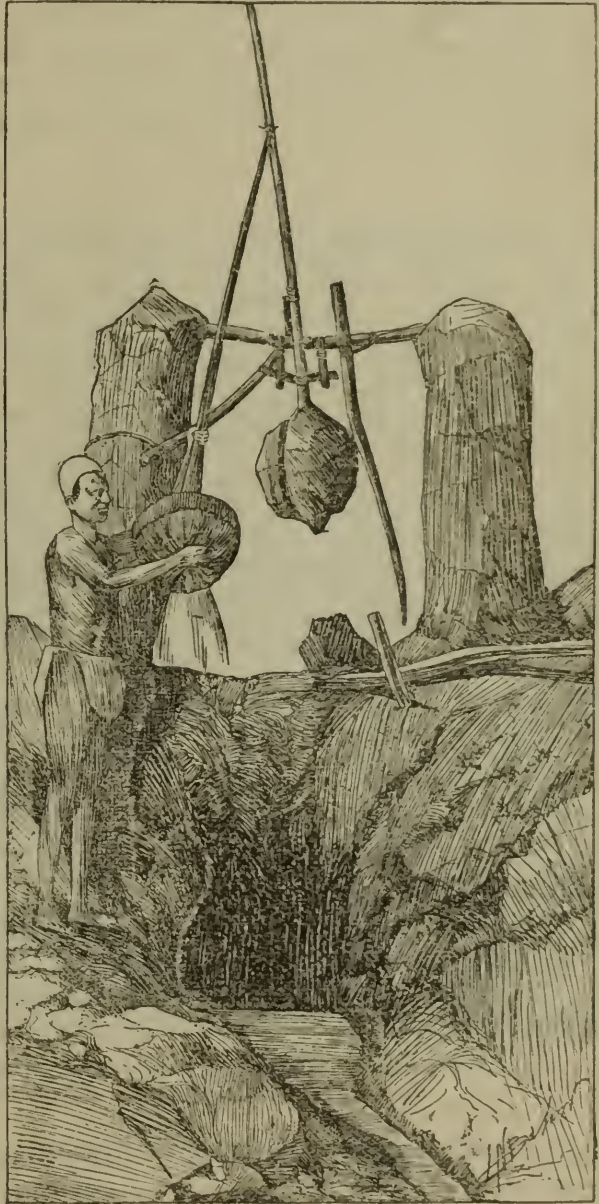
FIG. 47.—Shaduf, used in lifting water along the Nile and large irrigating canals in Egypt, with which water can be lifted 6 or 8 feet.
