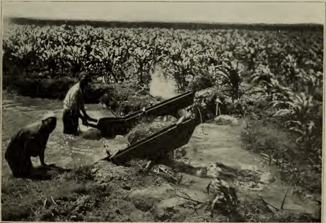
FIG. 2.—ROCKER FOR LIFTING WATER SHORT DISTANCES. [One of the many simple devices for irrigation in use in Egypt.]
