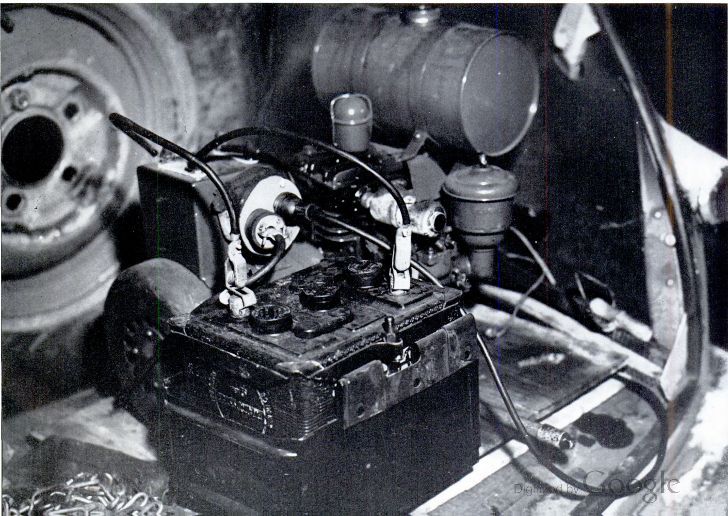
Below, Gasoline-driven generator in trunk of car used as power source in the field collection of air samples. Above, Automatic sulfur dioxide recorder in truck.
