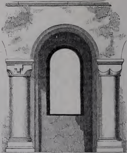
25. Chapel in the White Tower, London, A.D. 1081. Early Norman Arch and Window.
