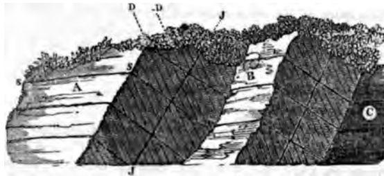
Stratification, joints, and cleavage.
