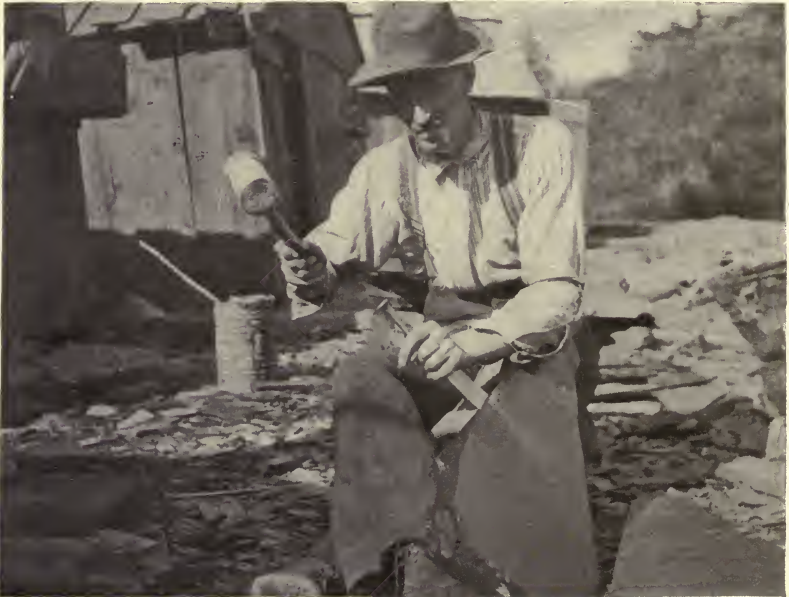
Fig. 20. — Slate dressing: splitting.
