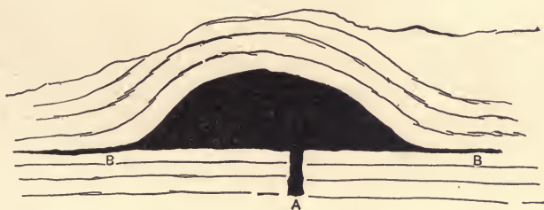
Fig. 10. — Laccolith, with supply neck (A) and sheets (B).
