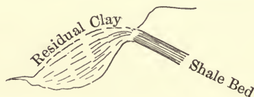
Fig. 26. — Effect of weathering on shale-limestone strata.
