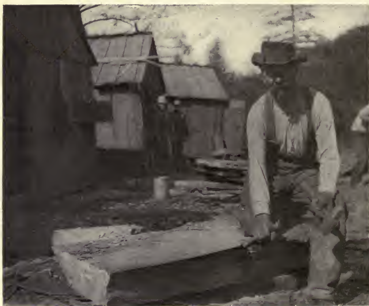
Fig. 18. — Slate dressing: the beginning of sculping.
