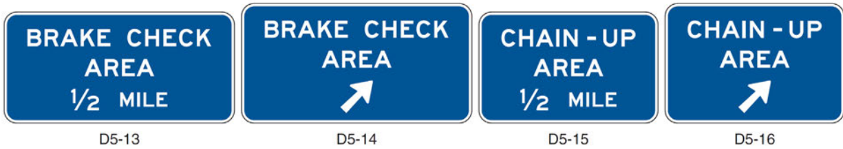
Figure 2I-6. Brake Check Area and Chain-Up Area Signs
