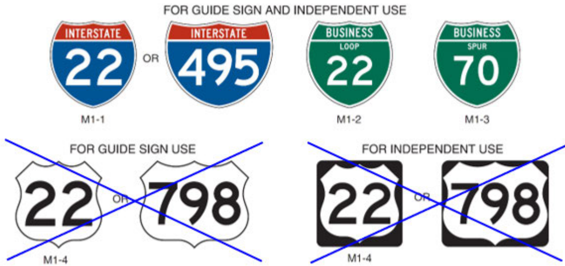
Figure 2E-17. Interstate, Off-Interstate, and U.S. Route Signs
