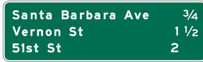
Figure 2E-31. Interchange Sequence Sign
