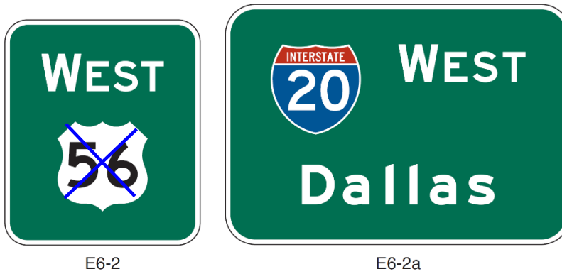
Figure 2E-2. Pull-Through Signs
