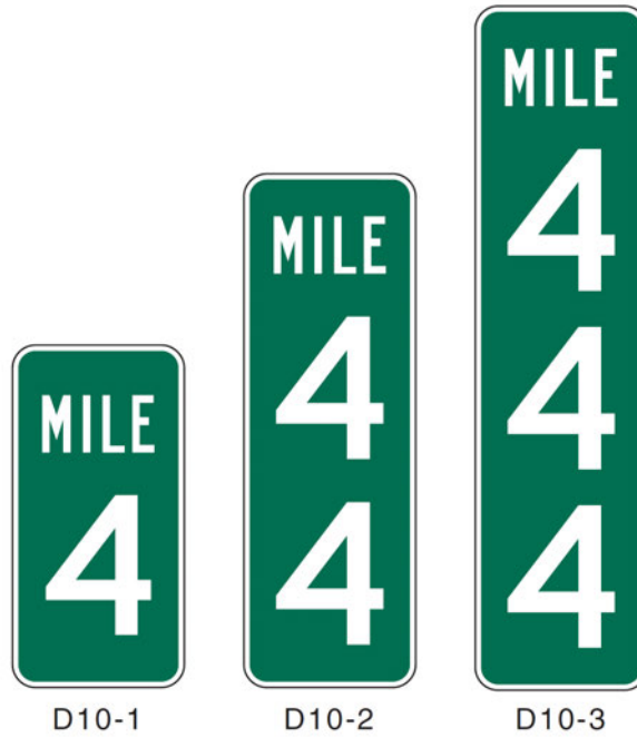
Figure 2H-2. Reference Location Signs
