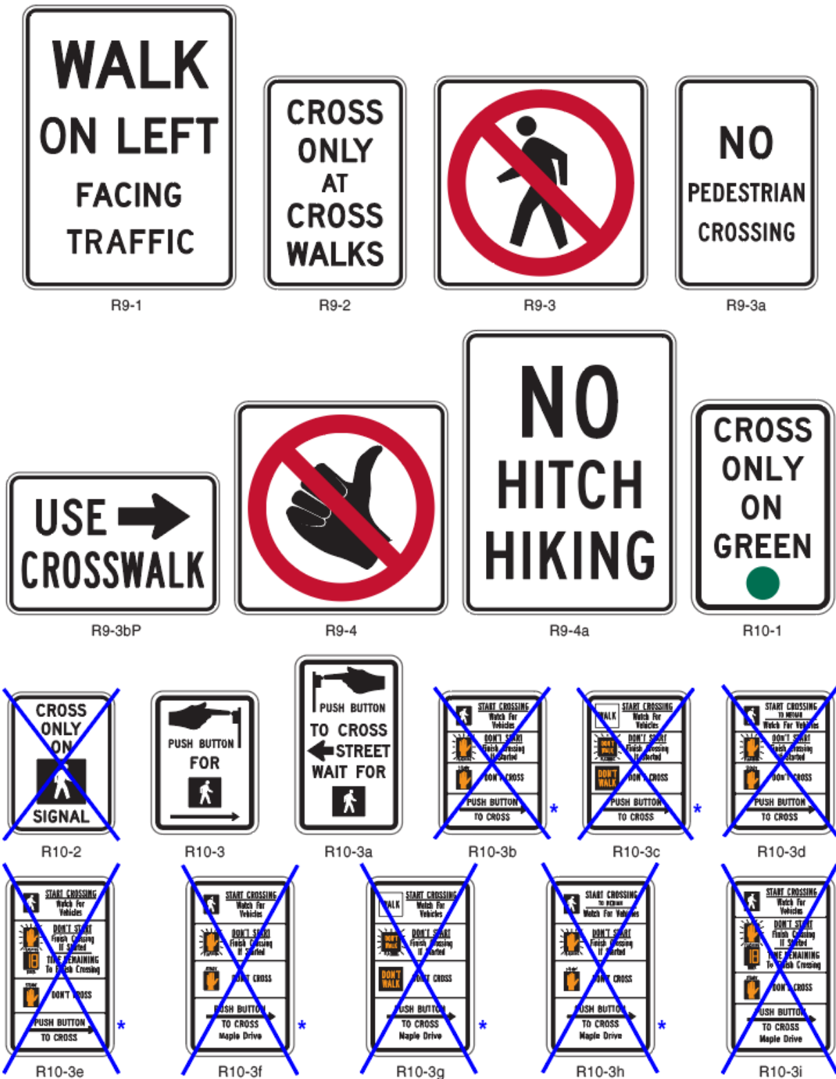
Figure 2B-26. Pedestrian Signs and Plaques (Sheet 1 of 2)
