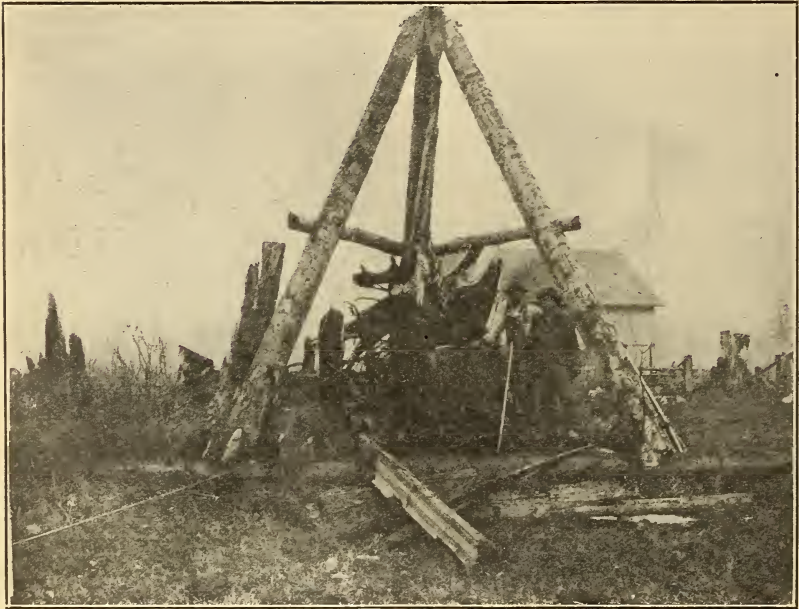
FIG. 11.—A stump puller that lifts the stump vertically out of the ground.
