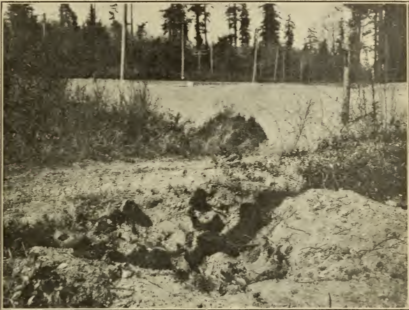
FIG. 25.—Roots left in the ground after a test stump had ceased to burn in a sandy soil. This has been advertised as a successful demonstration of char-pitting.
