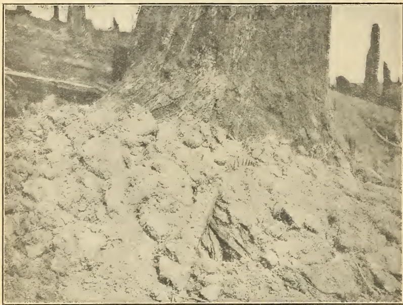
FIG. 21.—Char-pitting. Earth covering in place. Opening left at which to light the fire.
