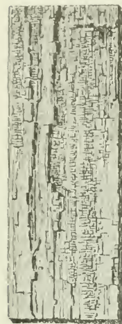
Fig. 493. Effect on wood of red spruce by the mycelium of Polyporus borealis . (Figs. 493, 494 are adapted from Bulletin No. 193, Cornell Experiment Station.)
