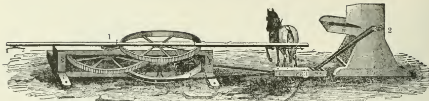
Fig. 112. A threshing device as pictured in 1845 (Warren's horse-power and thresher). "The machines may be placed as follows, viz.: The horse-power, Fig. 1, and the pulley-box, Fig. 3, outside the barn, and the threshing machine, Fig. 2, inside any convenient distance, say about 4 feet."
