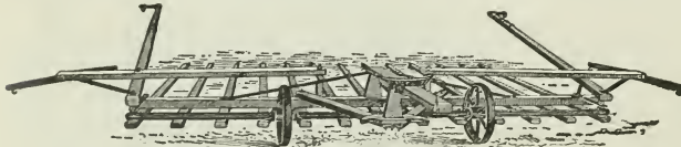
Fig. 128. A truss-frame sweep hay-rake.
