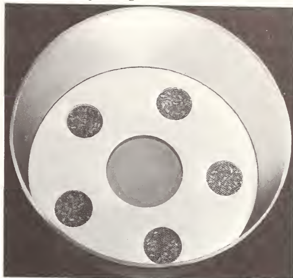
FIGURE 5.—A multichoice food preference chamber with samples from one untreated and four treated bins of grain sorghum.
