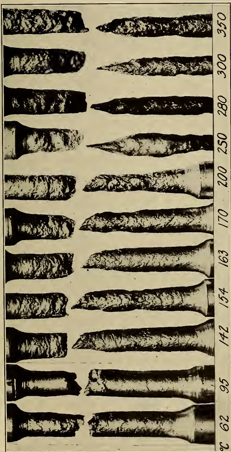
FIG. 4.—Tensile test specimens of pure zinc tested at elevated temperatures (second series) \times 1\frac{1}{8}
