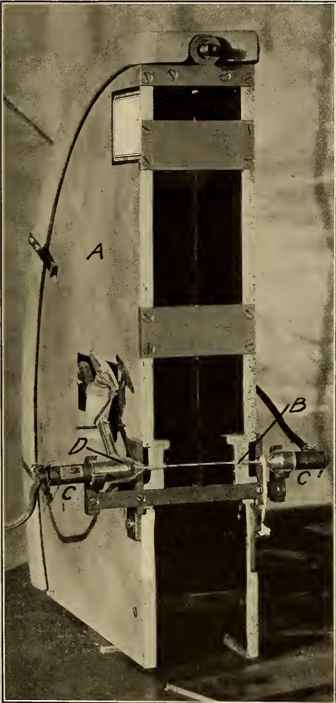
FIG. 16.—Cassette with device for heating specimens run at elevated temperatures
