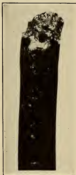
FIG. 14. — Orientation of cleavage faces in specimen 10 tested at 288° C.
