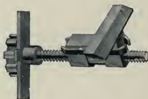
Fig. 4—Pull hook 8 ems long
