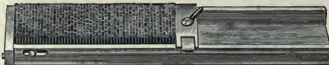
Shows the Galley locked at end and side
