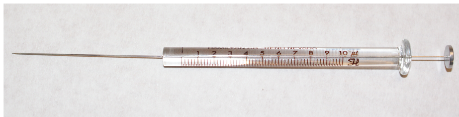
Figure 12.29 Example of a syringe for injecting samples into a gas chromatograph. This syringe has a maximum capacity of 10 \mu\text{L} with graduations every 0.1 \mu\text{L} .
