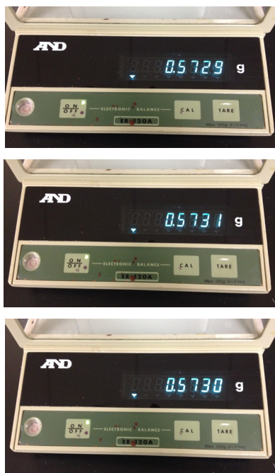
Figure 2.1 When weighing an sample on a balance, the measurement fluctuates in the final decimal place. We record this sample's mass as 0.5730 \text{ g} \pm 0.0001 \text{ g} .
