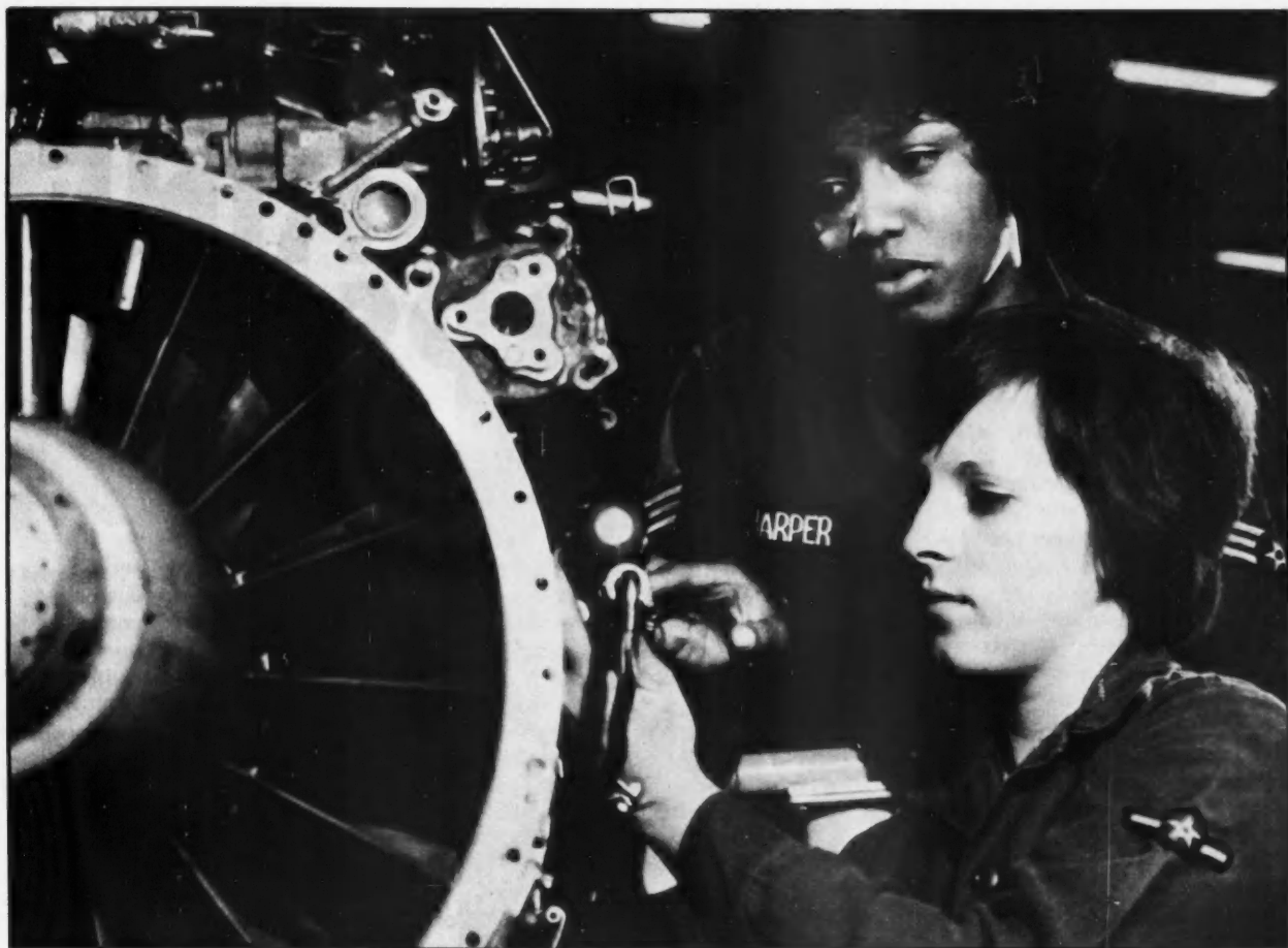
An Air Force sergeant (above) explains the installation of a fuel heater actuator valve on a jet engine to an airman trainee. Examining an Air Force patrol dog is one of the varied duties of women veterinarians in the Air Force.
