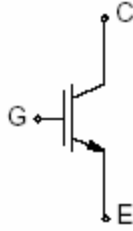
Figure 9. N-Channel IGBT Schematic Symbol [From Ref. 8].
