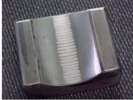
Figure 26. Bearing Race Fluting. [From Ref. 20].
