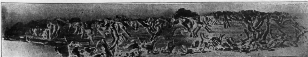
FIG. 10.—APPEARANCE OF TIMBER INFESTED BY CHELURA TEREBRANS.
