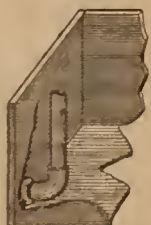
Fig. 5—Tank connection for drawing off juice
