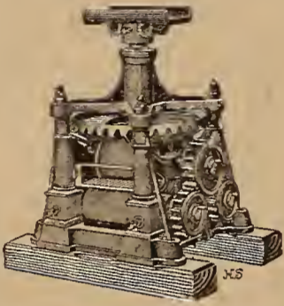
Fig. 2—Three-roller horizontal horse-power cane-mill
