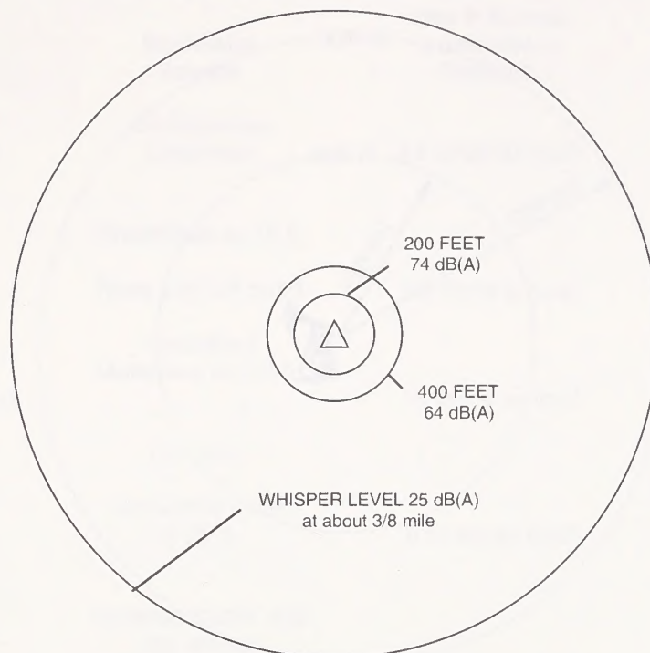
Illustration D-10 Average Envelope of Noise Levels Around a Drilling Rig
