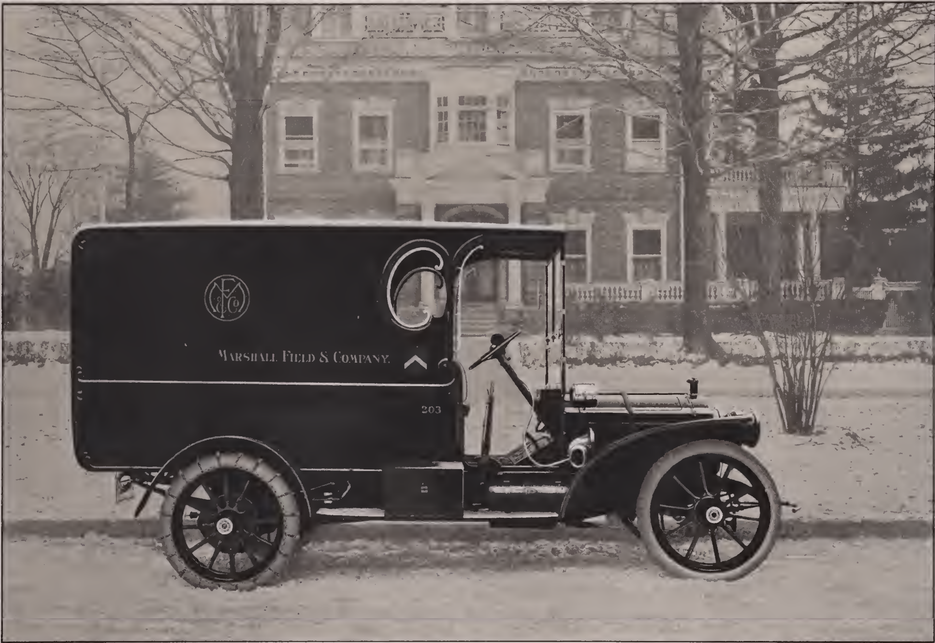
Fast light delivery body fitted to used Packard chassis
